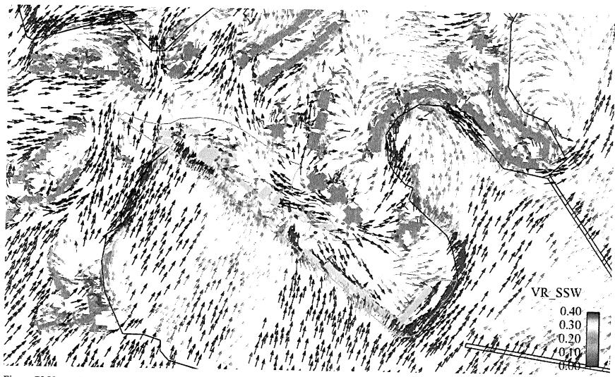
Figure C9 Vector Plot of VR under SSW Wind
