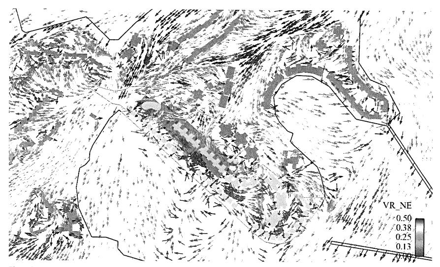
Figure C13 Vector Plot of VR under NE Wind
