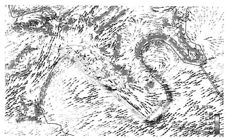
Figure C11 Vector Plot of VR under WSW Wind
