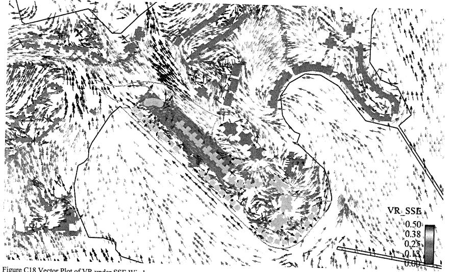
Figure C18 Vector Plot of VR under SSE Wind
