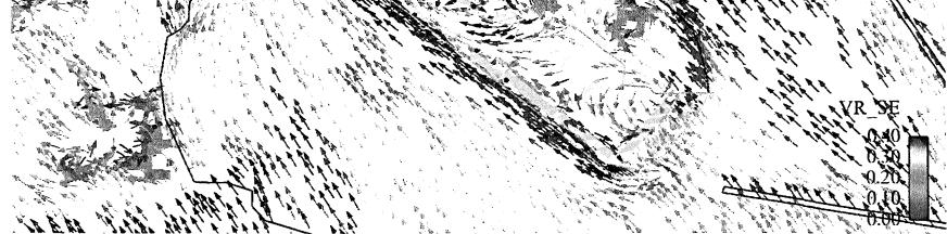
Figure C6 Vector Plot of VR under SE Wind
