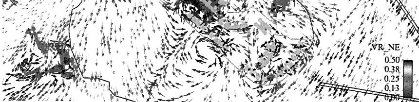
Figure C24 Vector Plot of VR under NE Wind
