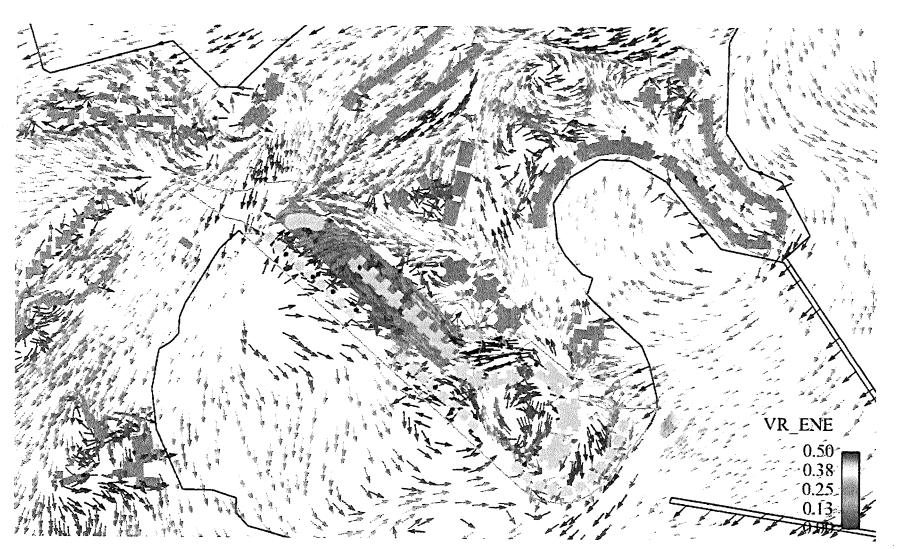
Figure C14 Vector Plot of VR under ENE Wind
