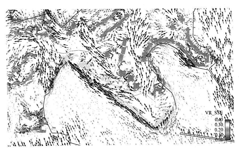
Figure C7 Vector Plot of VR under SSE Wind
