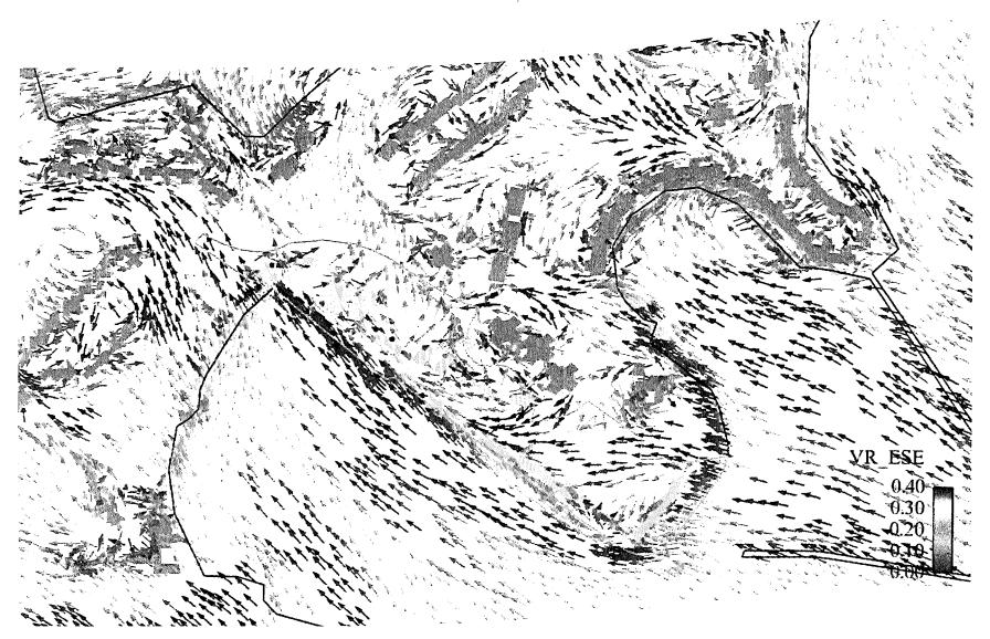
Figure C5 Vector Plot of VR under ESE Wind
